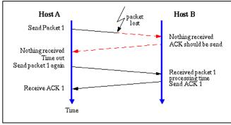
Figure A-10. Data transmission between two devices. [[25]
