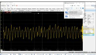
Figure A-31. The encoded signal at the output of our receiver's current feedback amplifier.
