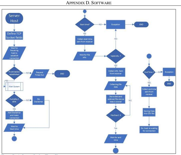
Figure D- 1. Server Socket Flow Chart
