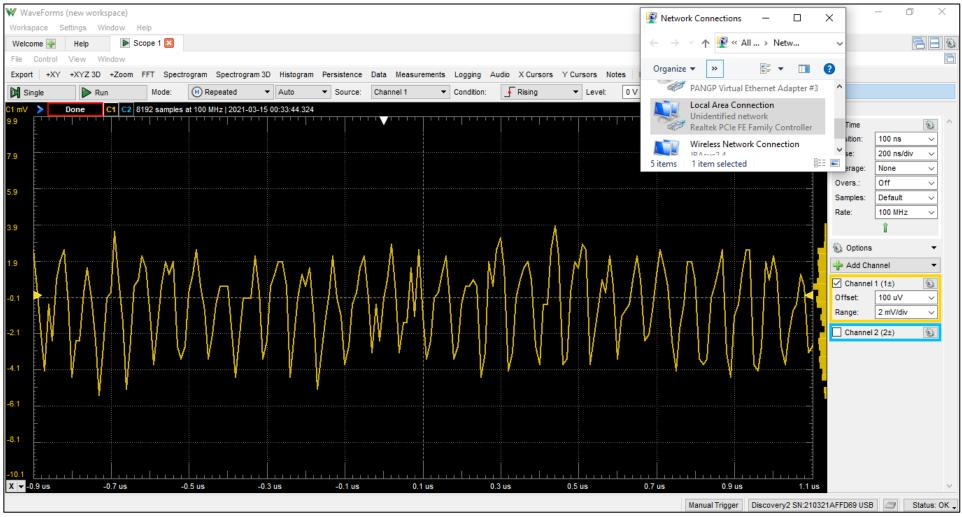
Figure A-31. The encoded signal at the output of our receiver's current feedback amplifier.
