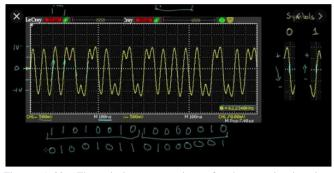
Figure A-30. Theoretical representation of ethernet signal using Manchester's encoding scheme. This image was captured from one of Ben Eaters YouTube videos. Check out his channel for all sorts of cool stuff. [[29]
