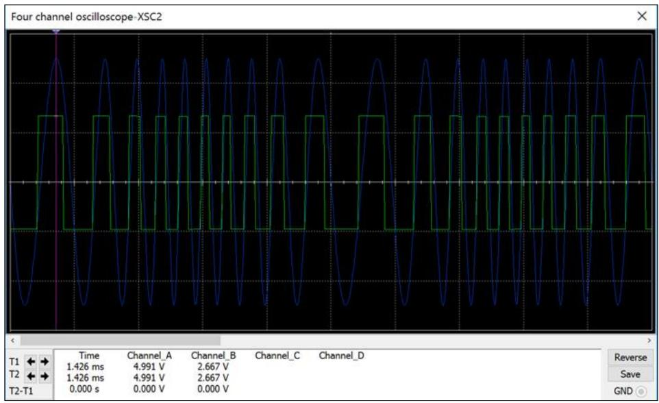
Figure A-24. FM Input Signal LT1713 Simulation Results.
