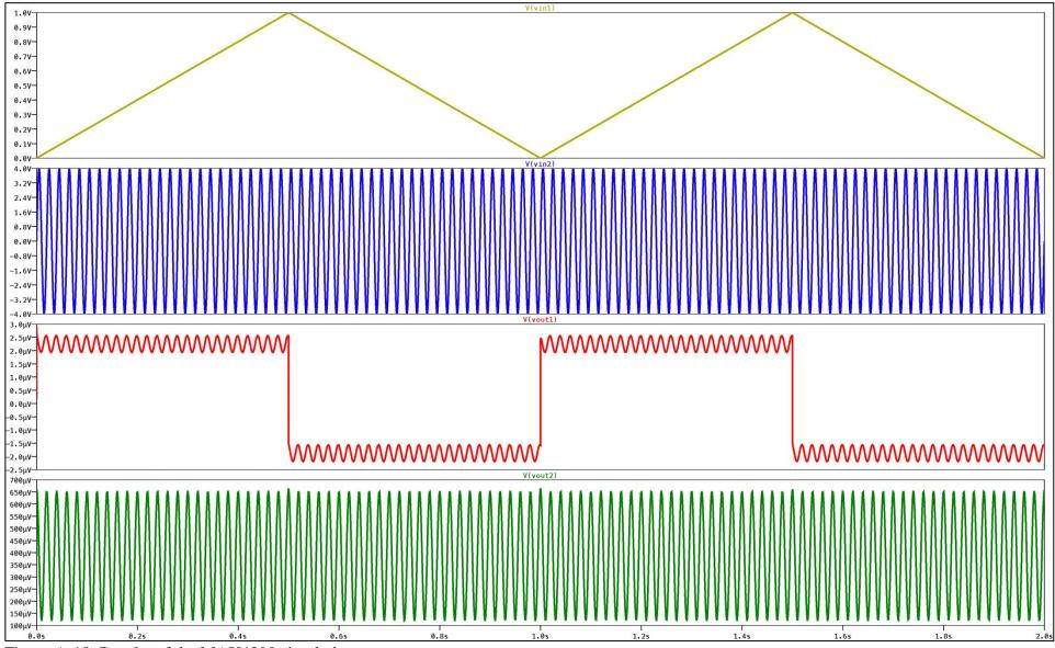
Figure A-18. Results of the MAX4390 simulation.
