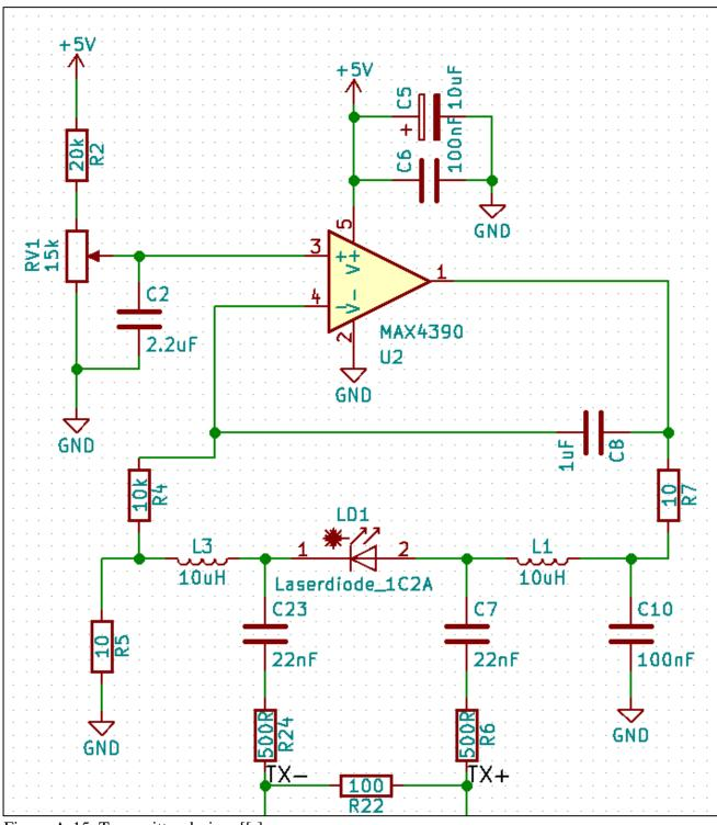
Figure A-15. Transmitter design. [[6]
