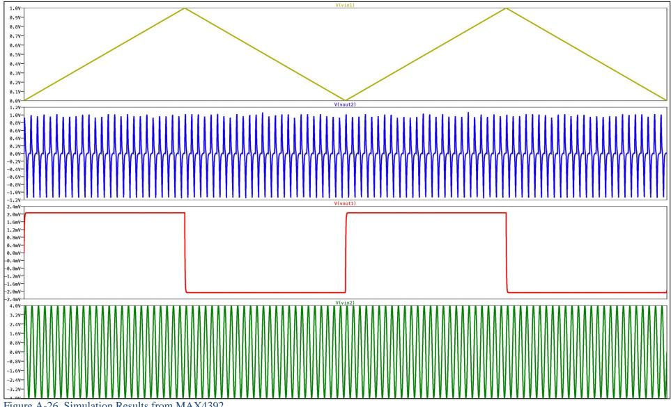
Figure A-26. Simulation Results from MAX4392.
