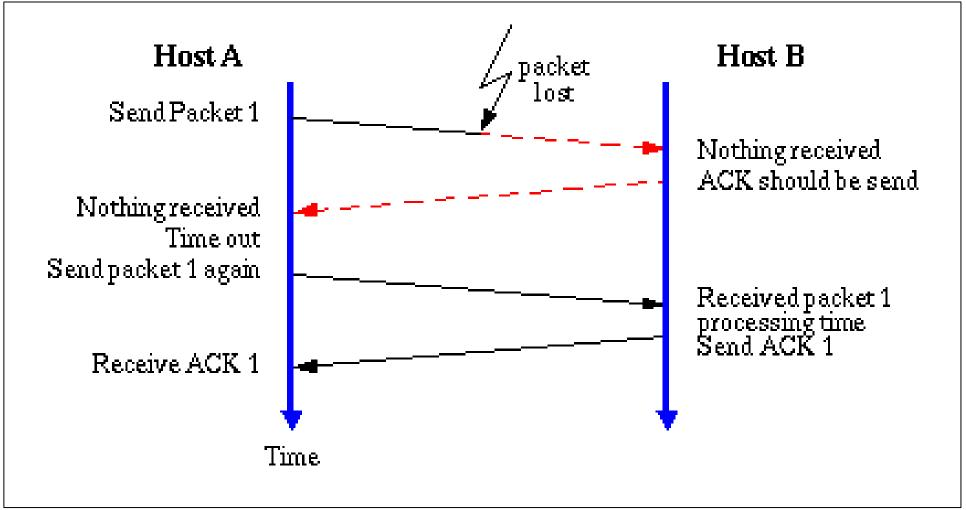
Figure A-10. Data transmission between two devices.
