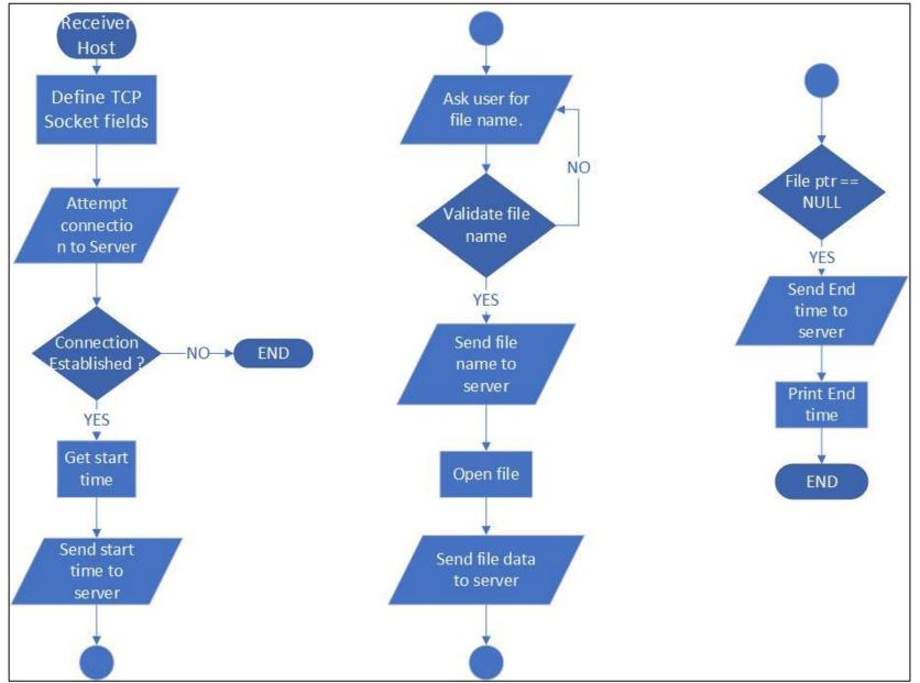
Figure D- 2. Client Socket Flowchart
