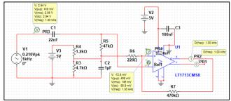
Figure A-22. LT1713 Op-amp design on Multisim.
